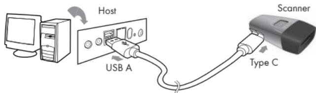
1. Flip open the Type-C USB port on the scanner.
