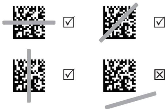
To scan a barcode, make sure the aiming beam fully covers the barcode.
