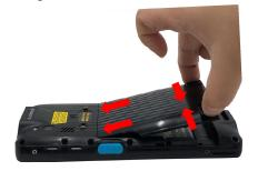
**3.** Press down the battery to secure in place.
